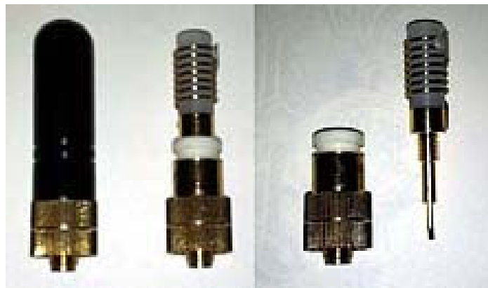
2" Stubby Antenna with only 1" of radiator Don't expect miracles.
